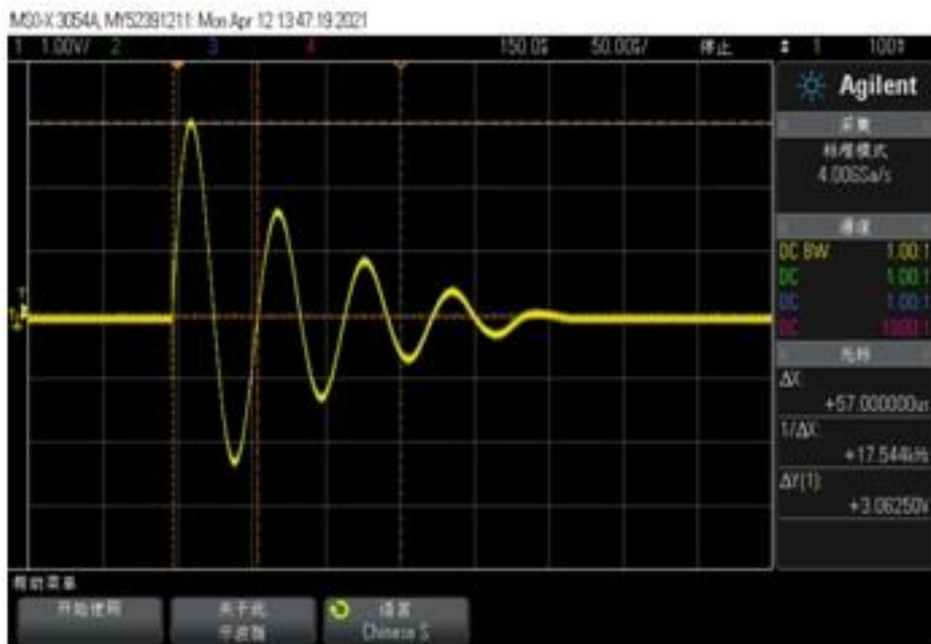
Typical Coil Current Waveform 306kA @ 17.544kHz
