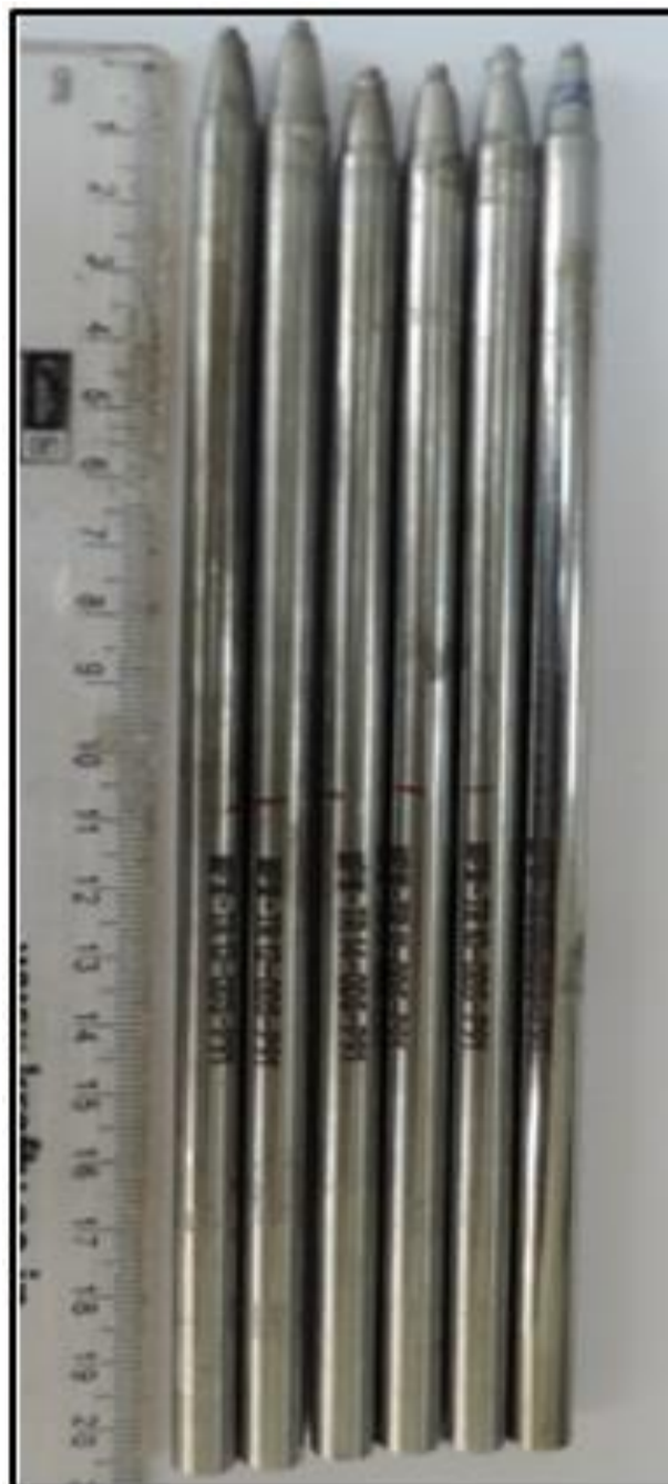
ODS clad tube to T91 end plug job post weld trial
