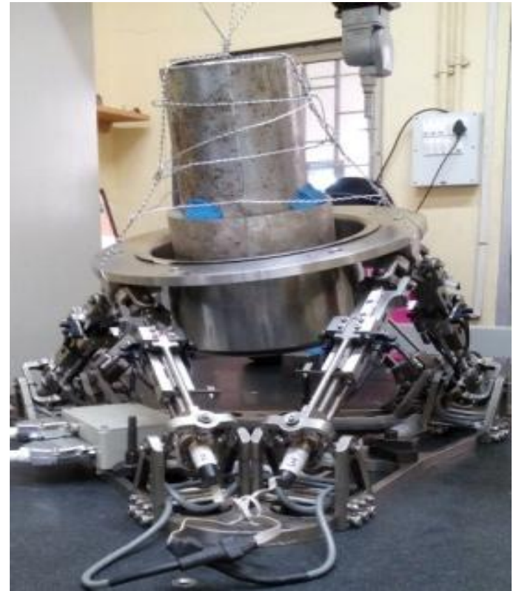
Mirror Positioning Mechanism System (MPMS) undergoing load test in CMM lab
