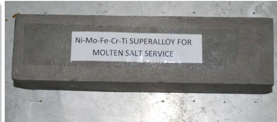
Air melted and investment cast alloy billet [in collaboration with MSD]
