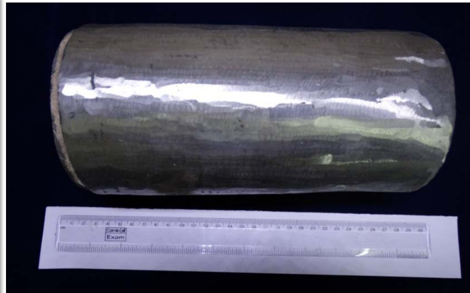
Billet manufactured by vacuum induction melting and casting [MIDHANI and MSD]
