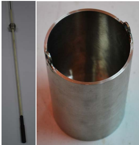
Electrode and Ni alloy crucible
