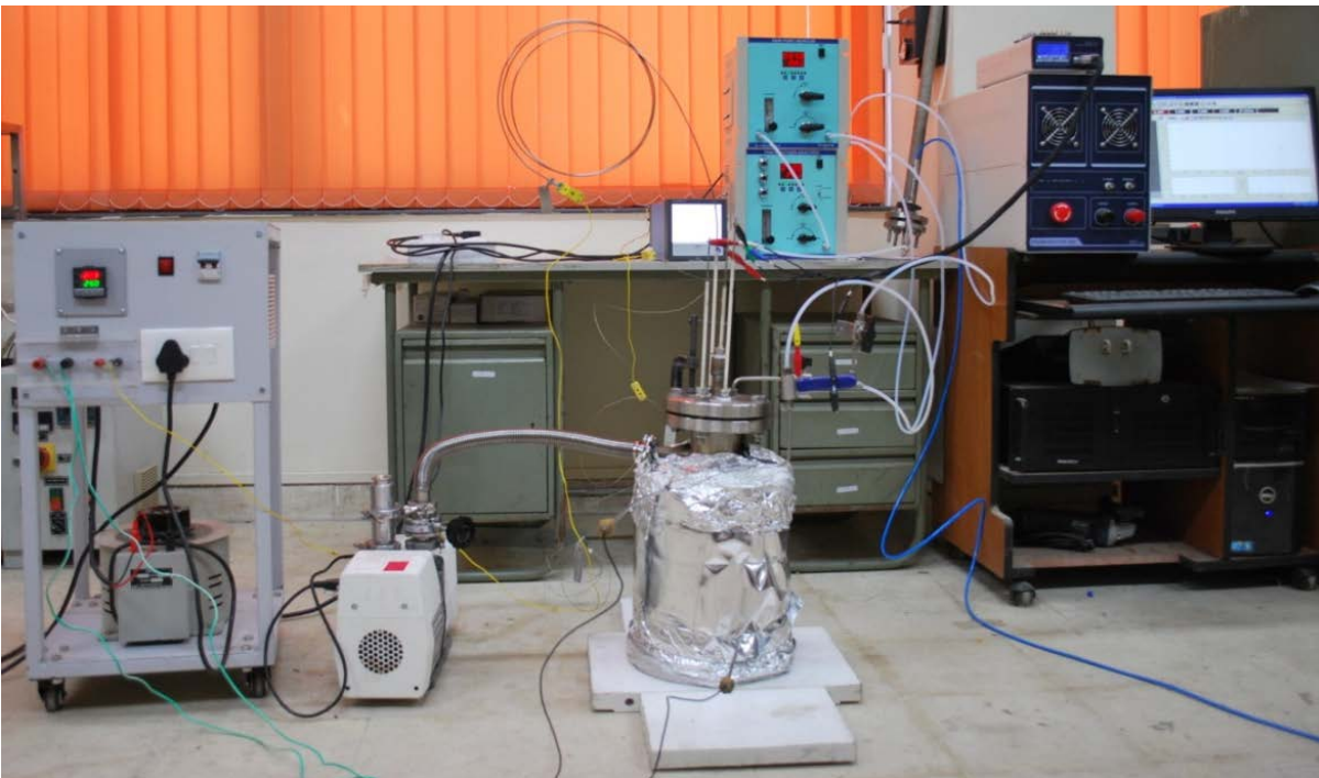
Facility for in situ determination of impurities along with data acquisition system
