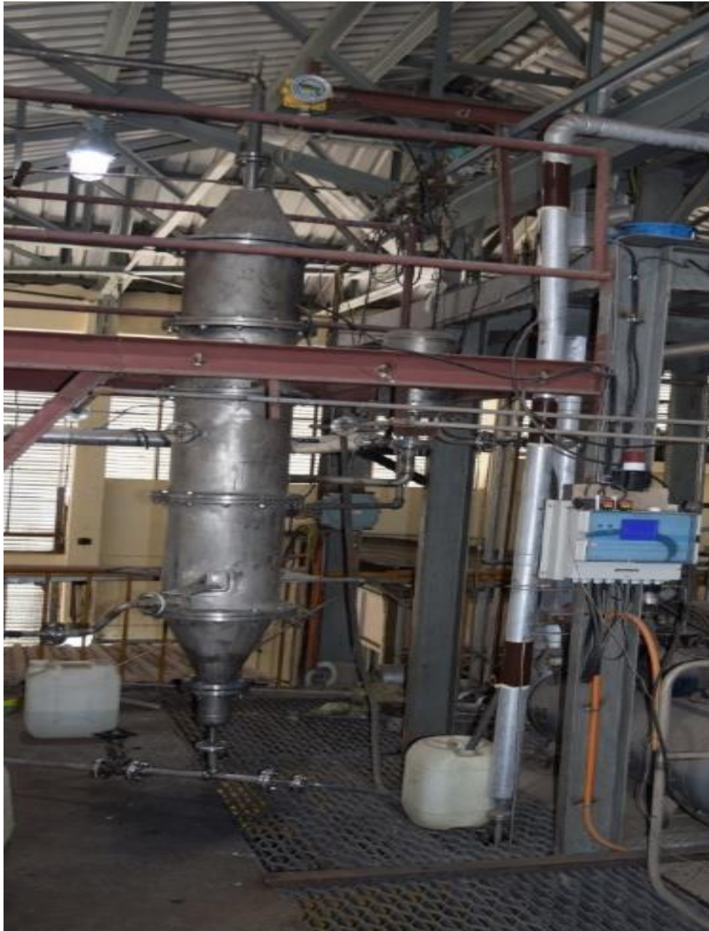
Experimental setup for adsorption of TCE on activated carbon using packed bed and its thermal regeneration.
