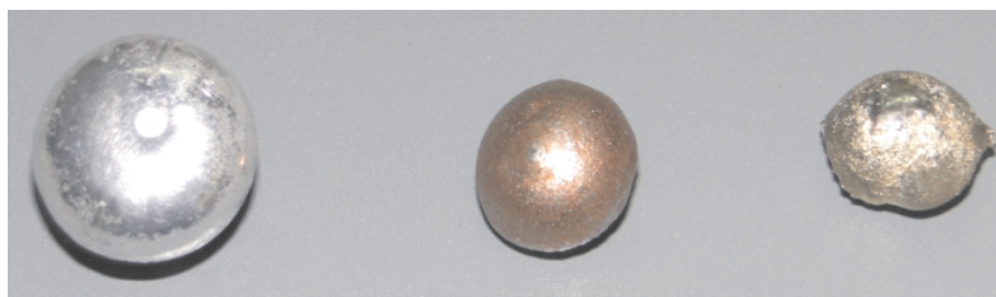
Fig. 7. Specimens of different metallic samples produced using ILM
