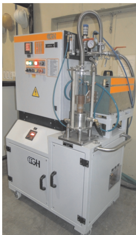
Fig. 4. Induction Levitation Melter (ILM) developed by NRG, BARC
