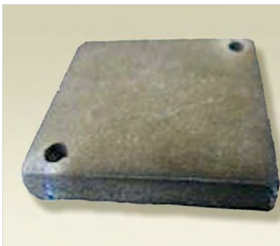
Fig. 4: Dense SiC coated C/C sample
