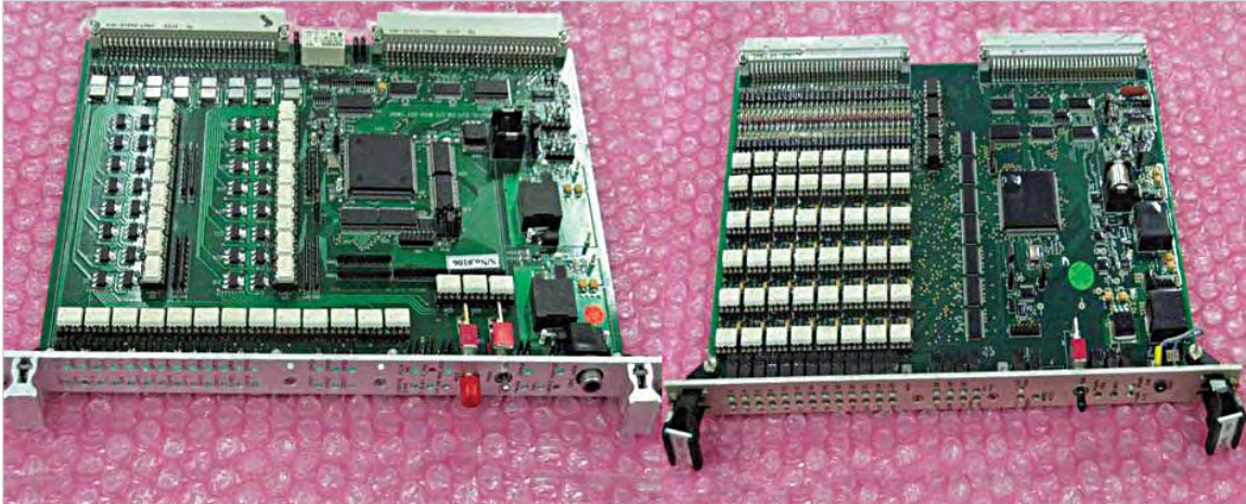
Fig. 2: Digital input and output boards
