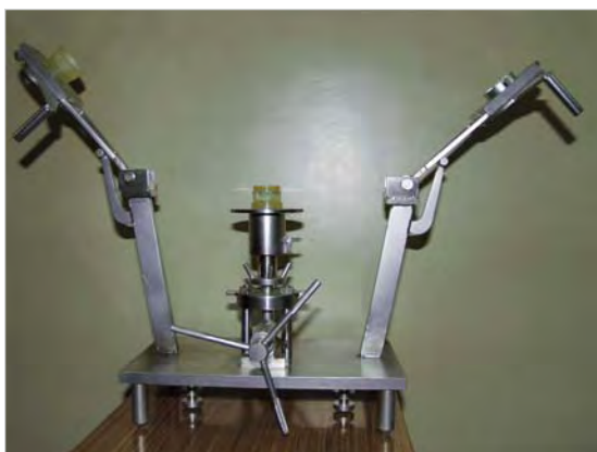
Fig. 2: Bottle double decapper for A3F, KARP
