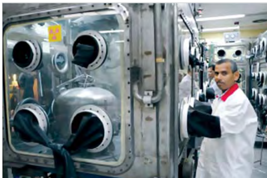
Fig. 3: Photograph of \text{U}_3\text{Si}_2 fuel granule production facility
