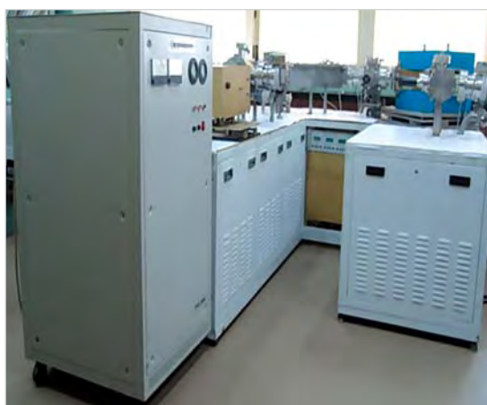
Fig. 18: Multicollector ICP – MS for RMP
