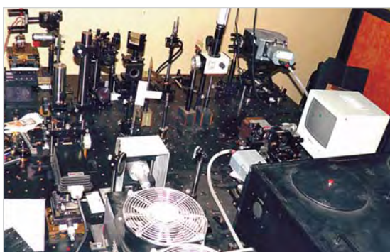
Fig. 5: Laser heated Diamond cell for high pressure high temperature measurements
