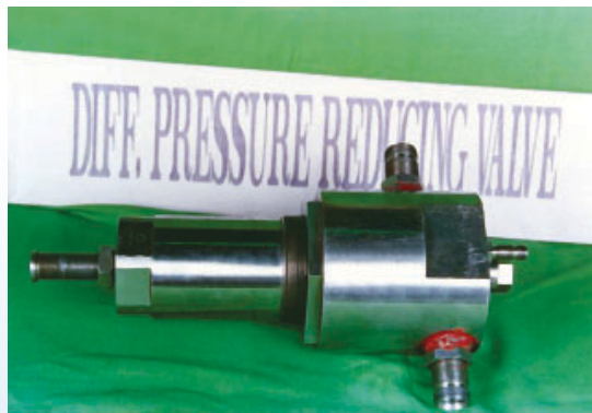
Fig. 2: High flow single stage DPRV
