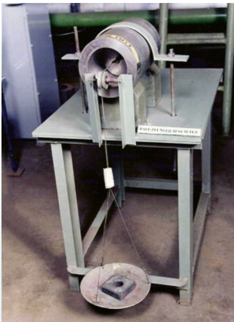
Fig. 9: Test set-up for vlier plunger
