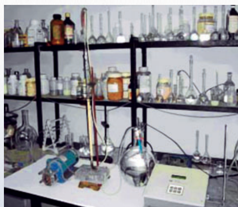
Fig. 1: Removal of Gadolinium Nitrate : experimental set-up
