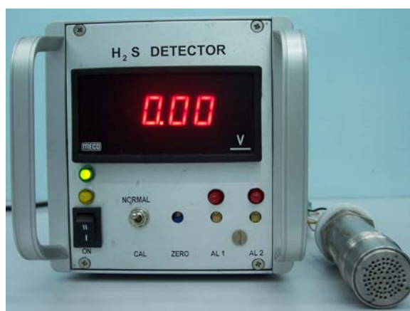
Fig.8: H_2S sensor connected to a monitor that has facility for calibration and provides alarms when the gas in the ambient exceeds pre-set limits
