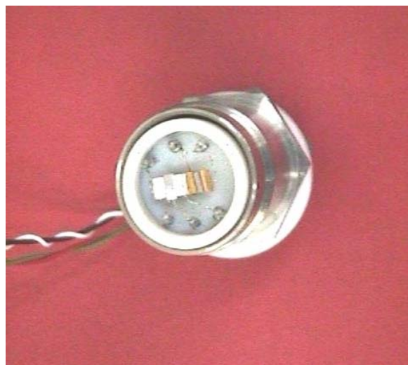
Fig.5: Photograph of \text{SnO}_2\text{:CuO} thin film based \text{H}_2\text{S} sensor showing heater and temperature sensor
