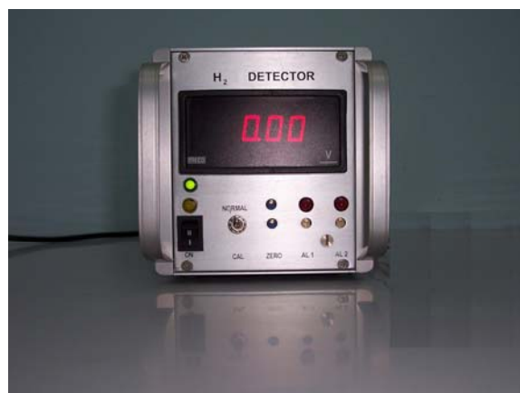
Fig.4: Instrument to detect H_2 in ambient that provides audio alarm when the gas exceeds a pre-set limit
