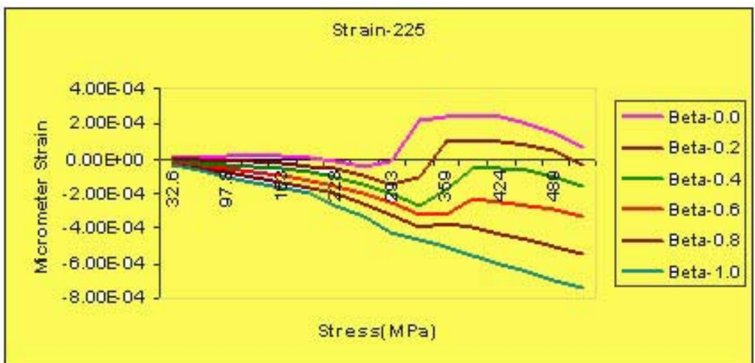
Fig 5 : Gauge location 225 Deg. & \beta = 0 to 1.0
