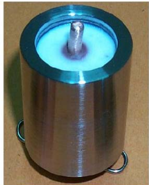
Fig.13. Photograph of LZS glass-ceramic to metal seal
