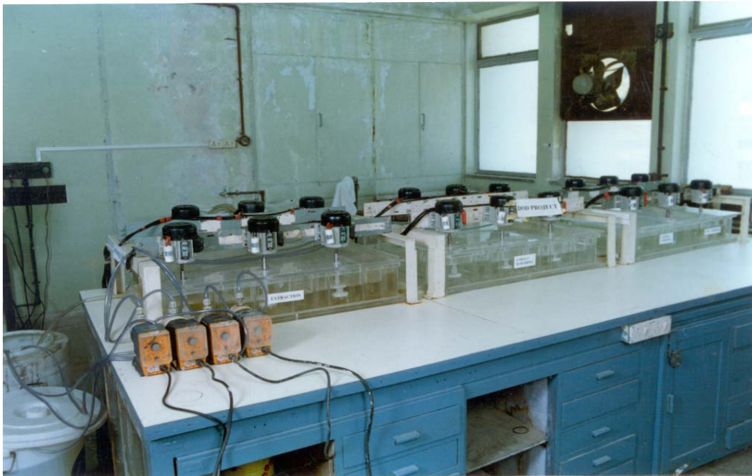
Fig.5 Acrylic mixer-settlers of 2.5 litres mixer capacity
