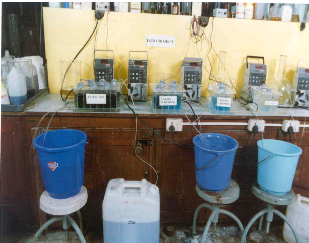
Fig.3 Laboratory setup of mini-mixer settlers
