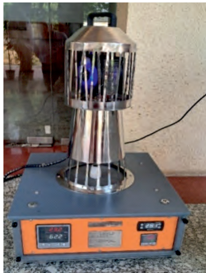
Air Moisture Collector commissioned at ESL in Kakrapar, Gujarat.
