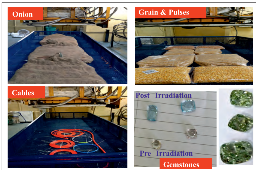
Radiation processing applications in 10 MeV, 3 kW accelerator at EBC, Kharghar.
