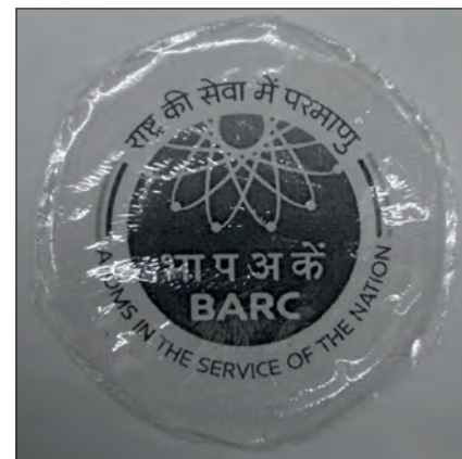
Plastic thin film detectors for real-time tritium detection.
