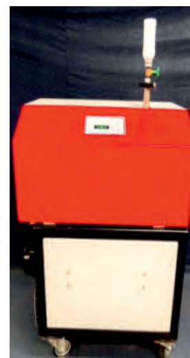
He Leak Detector.
