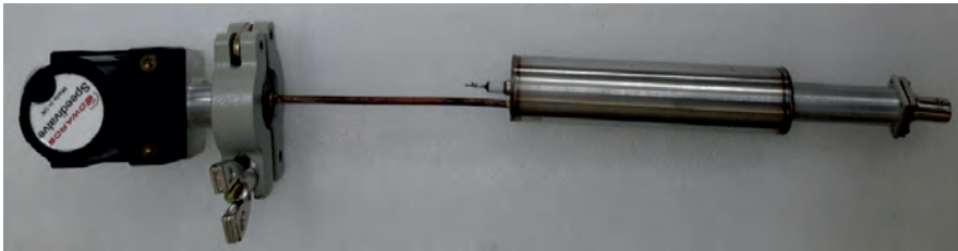
Natural boron coated proportional counter employing dip coating method.
