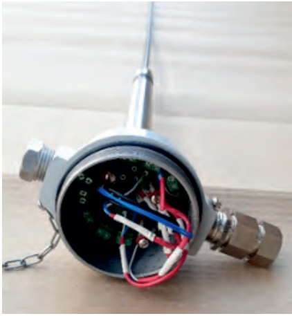
Small Scale prototype level sensor with standard sensor head.
