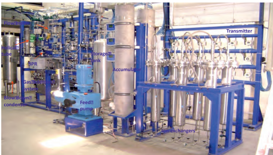
Normal temperature Equipment/components of a test facility established for carrying out experimental validation of CLOE.
