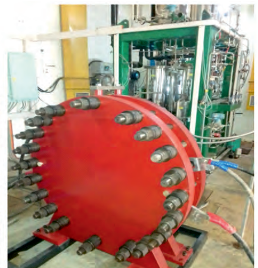
Left to Right: 50kW Electrolyser cell module; and prototype to 0.5MW cell, integrated with the plant.
