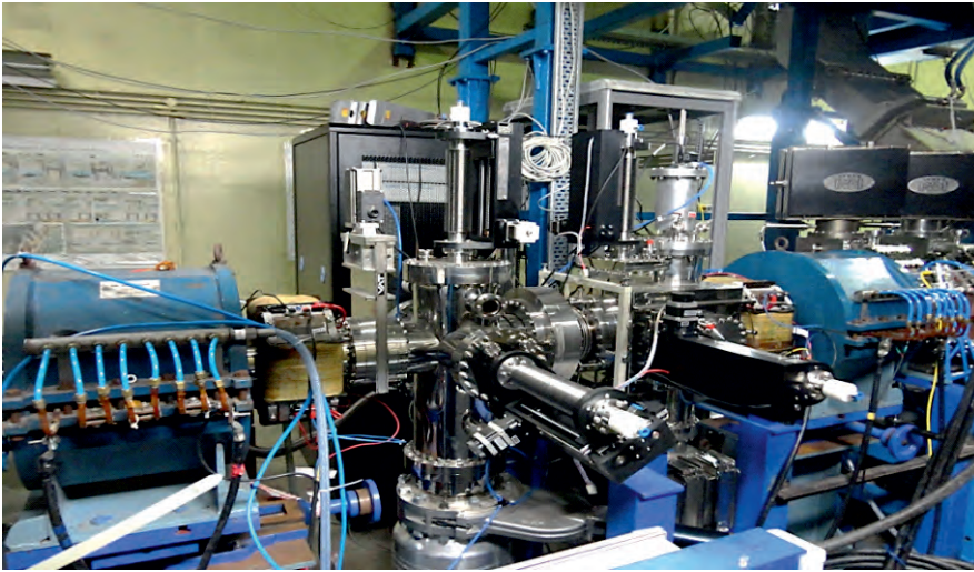
Two-solenoid based LEBT Line in LEHIPA.
