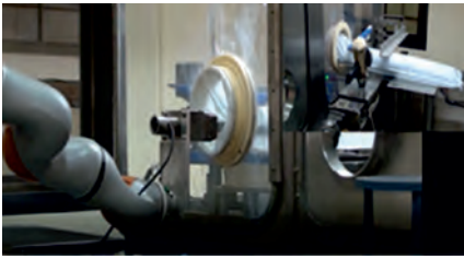
Robot performing the bag-in operation.
