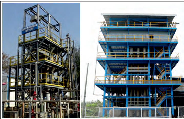
Left to Right: Radiotracer experiments in a cross-flow reactor; and in a pulsed extraction column.
