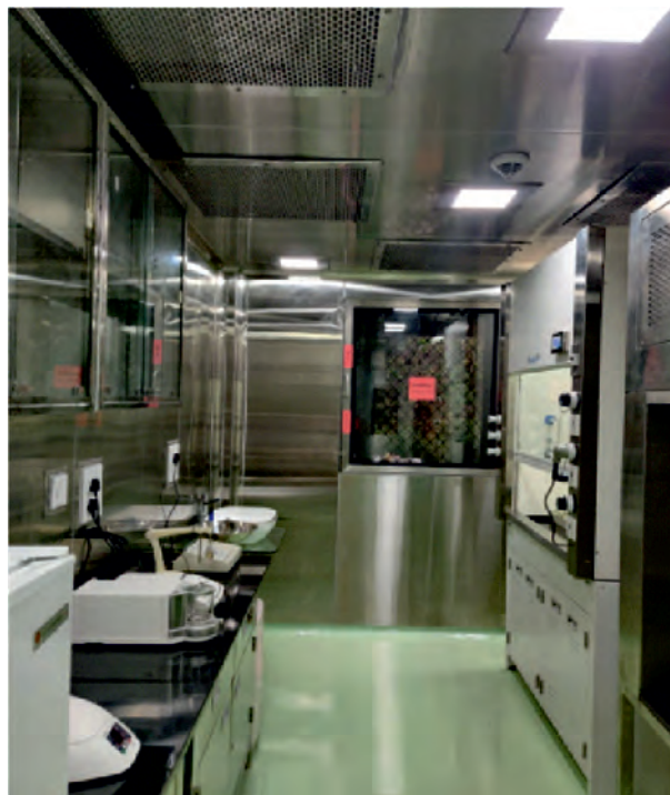
Clean room facility of Class 10,000 with fume hood and Clean Bench of Class 100 for sample processing for ultra - trace analysis (EMAD Laboratory at BARC Hospital).
