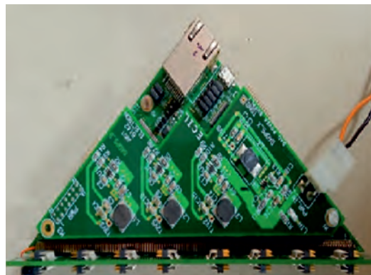
128-channel DAQ system.
