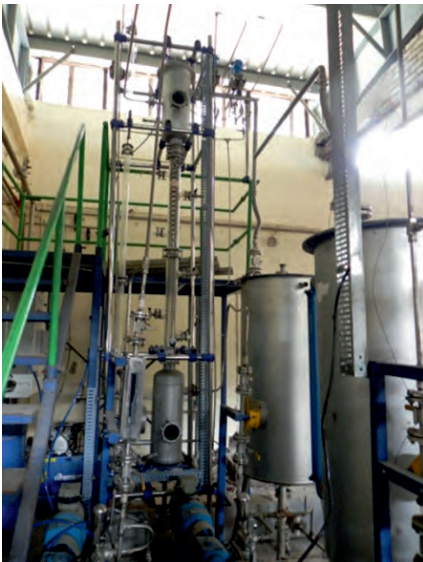
Pulsed Disc and Doughnut Column (PDDC) demonstration setup at Uranium Extraction Division in BARC.
