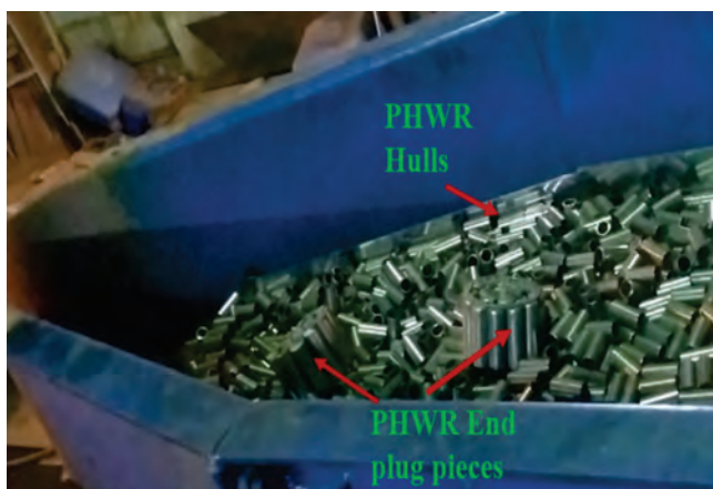
Fig. 14: Batching of PHWR Hulls with End plugs
