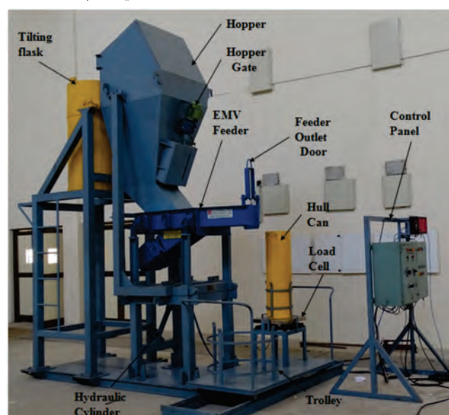
Fig.1: Batching System installed at Test Facility, Kalpakkam
