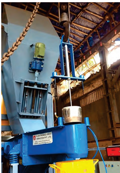
Fig. 9: Remote handling of Feeder Gate
