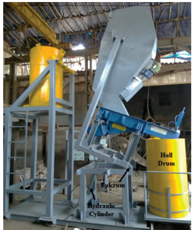
Fig.11: Emergency Hull Draining operations
