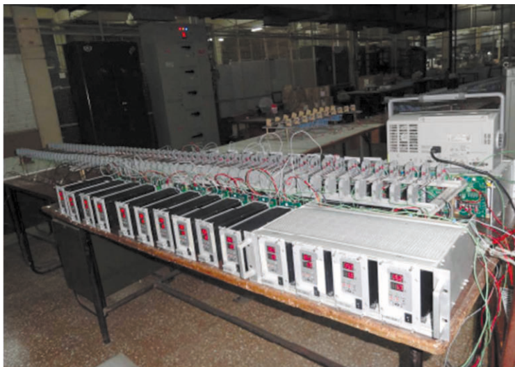
Fig. 8: Latest embodiment of ECPS SM100 fourteen of them sharing the load
