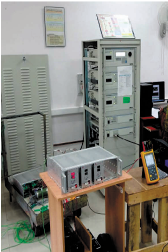
Fig. 6: The Power Quality Testing Equipment Connected to ECPS (left showing testing of single ECPS unit, right showing the testing of Multiple ECPS units)
