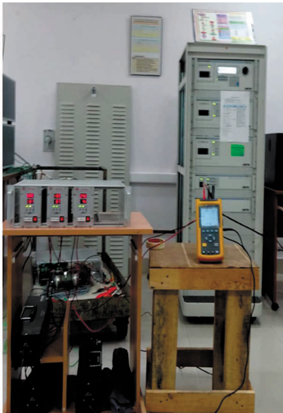
Fig. 6: The Power Quality Testing Equipment Connected to ECPS (left showing testing of single ECPS unit, right showing the testing of Multiple ECPS units)
