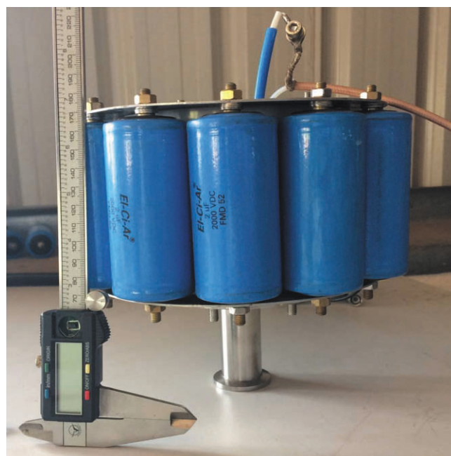
Fig. 6: Photograph of miniature plasma focus based pulsed neutron generator.
