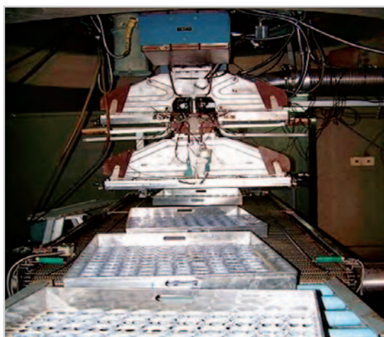
Fig.2: PE O rings being irradiated
