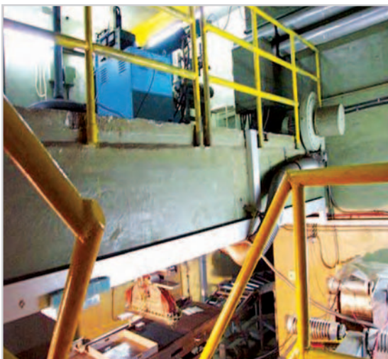
Fig.1: A view of the irradiation cell (top: RF Cavity; bottom: irradiation area with conveyor)
