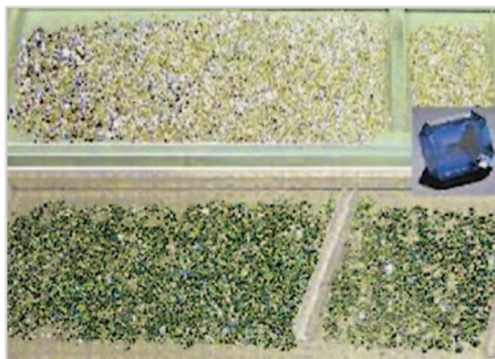
Fig.5: Unirradiated diamonds(Top); Colored Diamonds (Bottom) by EB irradiation
