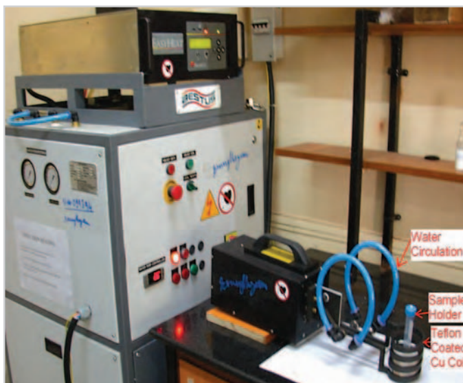
Fig. 3: Induction heating system
