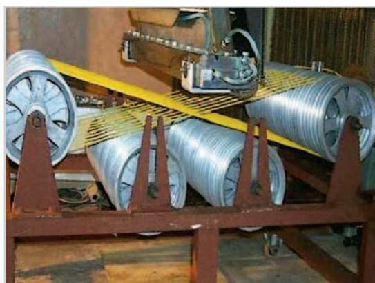
Fig. 4: Irradiation set up used for cable treatment
