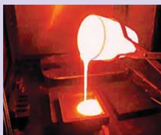
Fig. 4: Pouring of molten vitreous mass in laboratory
