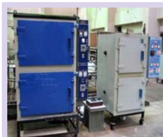
Fig. 9: Thermal ageing test chambers
