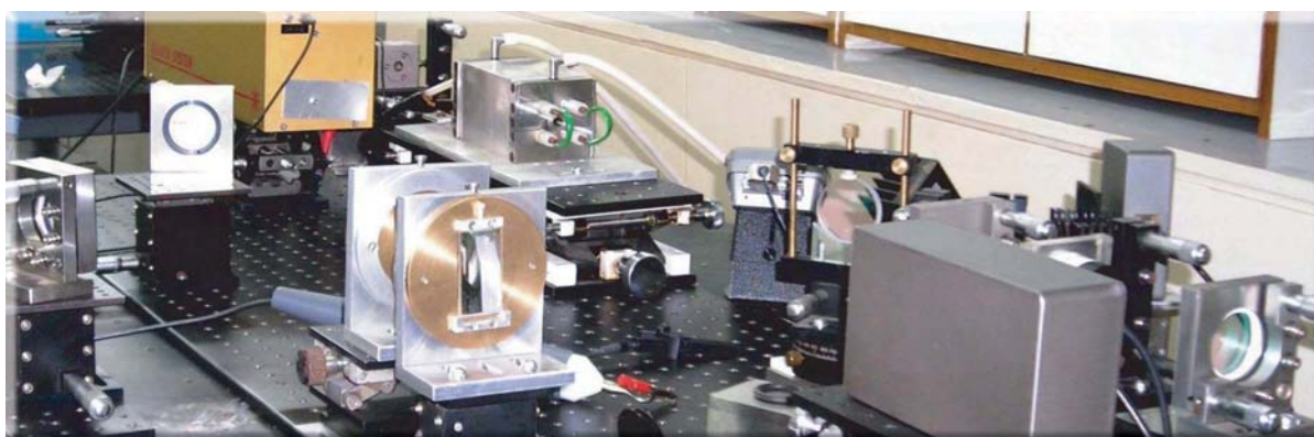
Fig. 5: The regenerative amplifier assembly with two cylindrical lenses in the foreground. The Nd:Glass rod enclosed in an aluminium reflector, the two pockels cells with their respective 3.5 KV pulse generators
