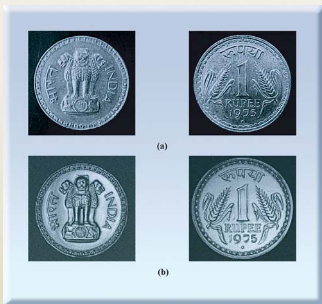
Fig. 7 : (a) Digital photo and (b) Ultrasonic C-scan image of an Indian coin
