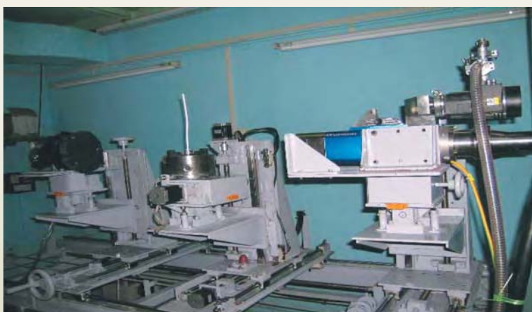
Fig .1 : Experimental set-up for phase-sensitive imaging experiments
