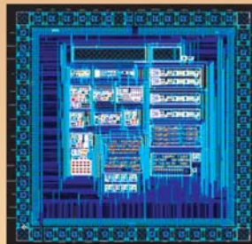
Anu-Shikhar: First prototype Low power peak detect & hold
