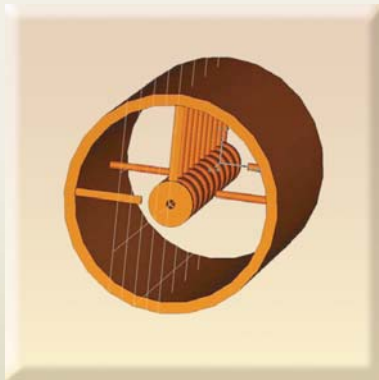
Fig. 5: Model of post couplers in DTL
