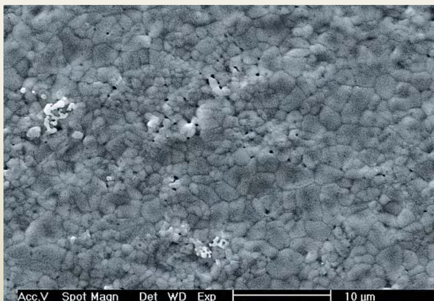
Fig. 3: SEM micrograph of RE 2 O 3 pellet sintered at 1200°C for 2 h.
