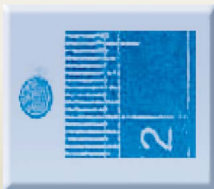
Fig. 10 : Small punch test specimen (3 mm diameter)
