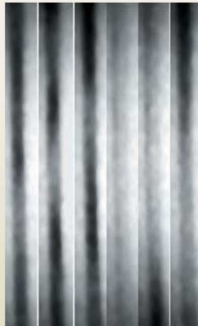
Fig. 24: Images of mixture of air and of water inside metal tube (dark shades indicate water)
