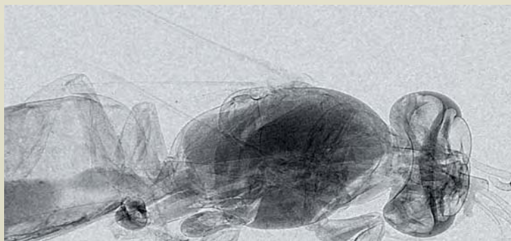
Fig. 4 : Image of a bee taken in phase radiography mode (microfocus source)
