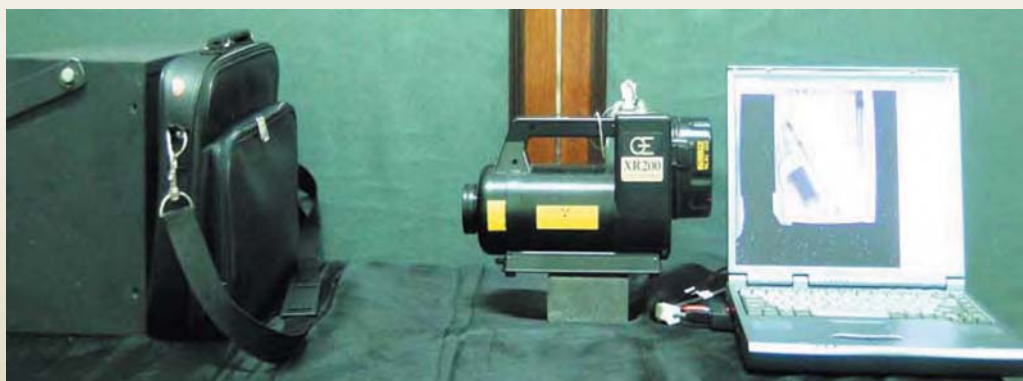
Fig. 17 : Photograph of portable baggage inspection system
