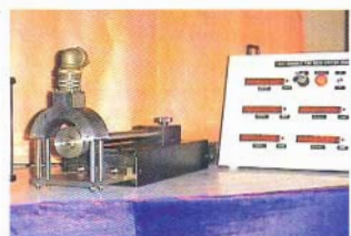
Test Console for qualification of Reed Switch Assembly
