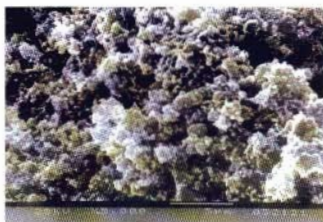
Fig. 6 : SEM picture of \text{Pd}_{17}\text{Se}_{15} obtained from [\text{PdCl}(\text{SeCH}_2\text{CH}_2\text{NMe}_2)(\text{PPh}_3)]
