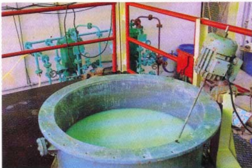
Fig. 3 : Agitation tank used for ^{232}\text{Pa} recovery plant
