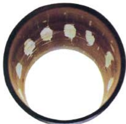
Fig.3: Multiple scraped locations inside a tube
