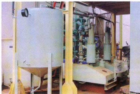
Fig.4 : Vacuum station used for 231 Pa recovery plant
