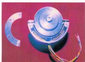
Reed Switch Assembly - before potting
