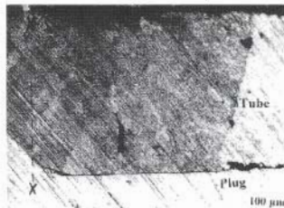
Fig. 3 : A centre-line crack in one of the laser welds made at laser power = 900W & welding speed = 20 rpm
