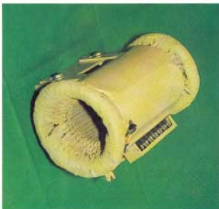
Fig.8 : Magnetic steerer designed and built for FOTIA beam line
