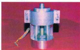
Fixture for checking actuation of Reed Elements
