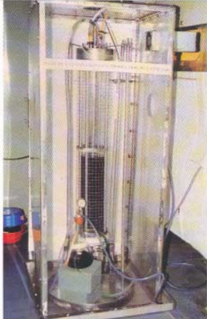
Pilot plant for uranous nitrate production by catalysis
