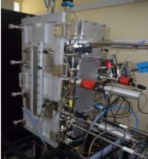
Indigenously developed Sputter Coating Machine for Metal Membrane Fabrication
