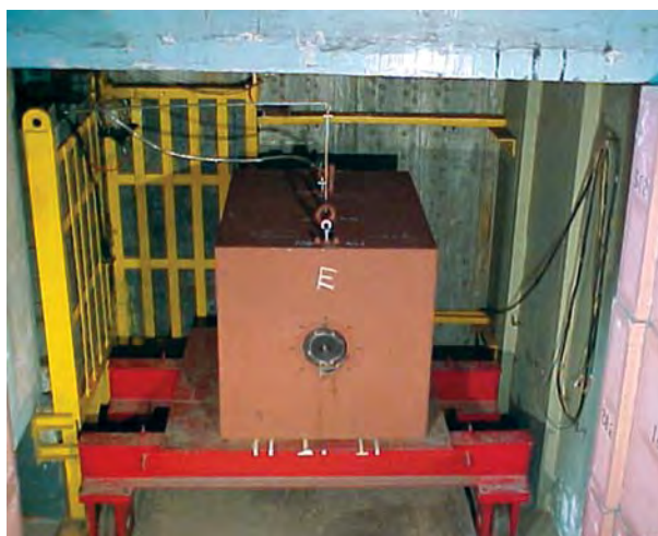
Shielding Corner Facility with AHWR Shield Model on Trolley
