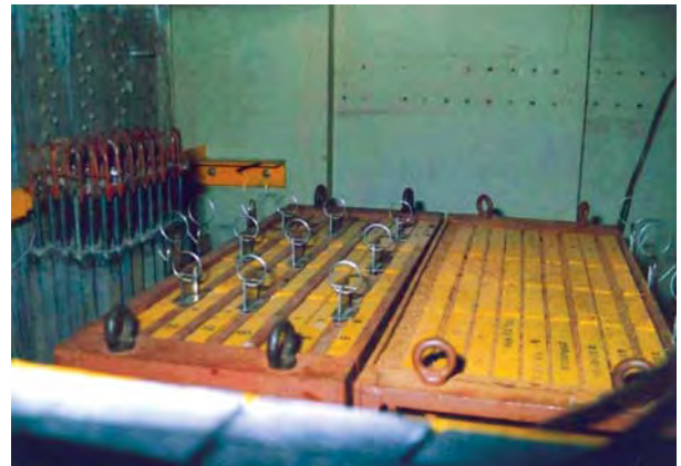
A Typical Arrangement of PFBR Shielding Experiments at Apsara
