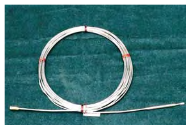
Source Range Monitor
