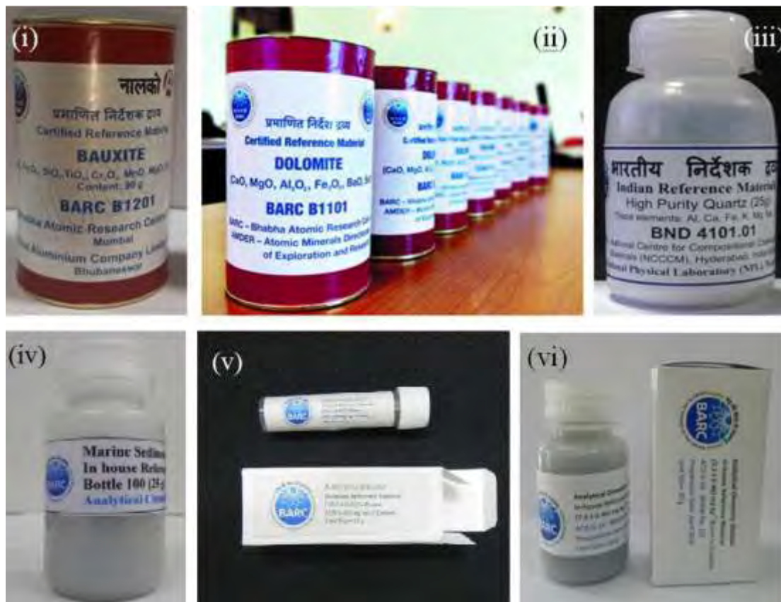
Fig. 1: Photographs of CRMs/in-house RMs: (i) Bauxite (BARC B1201) (ii) Dolomite (BARC B1101), (iii) Quartz (BND 4101.01), (iv) Marine sediment (ACD-MS-01), (v) Zirconium boride (BARC/QCM-ZrB 2 /2023), (vi) Graphite for boron (ACD-G-16)
