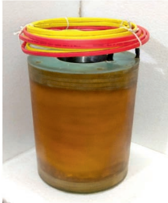
Figure 17.4. Magnetic coil for X-band BWO.
