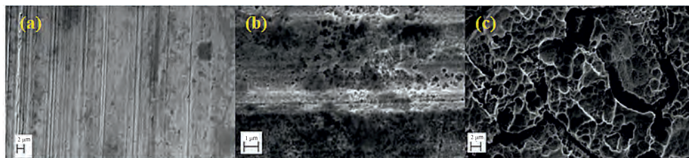
Figure 25.7: SEM images showing comparison of Ta substrates before and after etching in different conditions: (a) before etching, (b) etching without O_2 , and (c) etching with O_2 .
