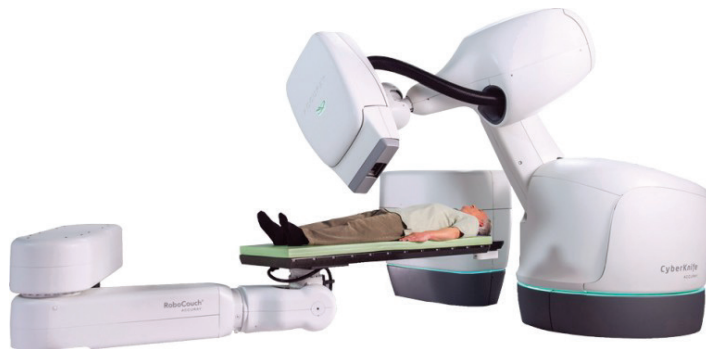
Figure 29.1: CyberKnife: A linac based radiation delivery system [145].
