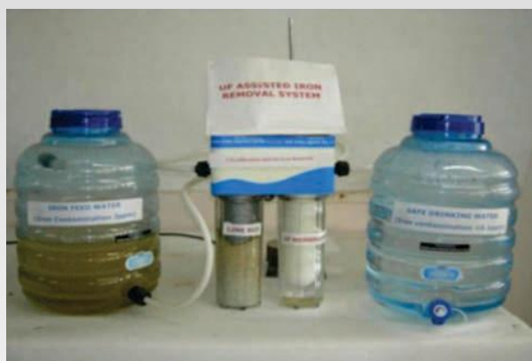
Domestic Water Purification Unit for Iron Removal
