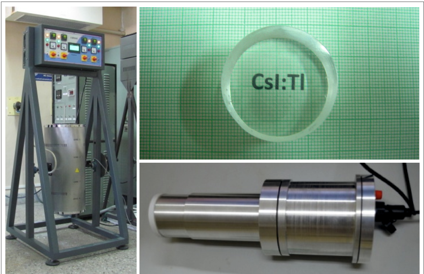
Fig.1: Photograph of (a) Bridgman Crystal Growth Furnace at TPD, BARC. (b) Processed CsI:Tl single crystal and (c) A typical radiation detector based on CsI single crystal.
