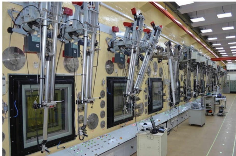
Fig. 1: Operating area of the hot cells in the NHF showing the viewing windows and master slave manipulators
