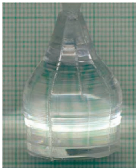
Fig. 1: As-grown LTB:Ag crystal ingot.
