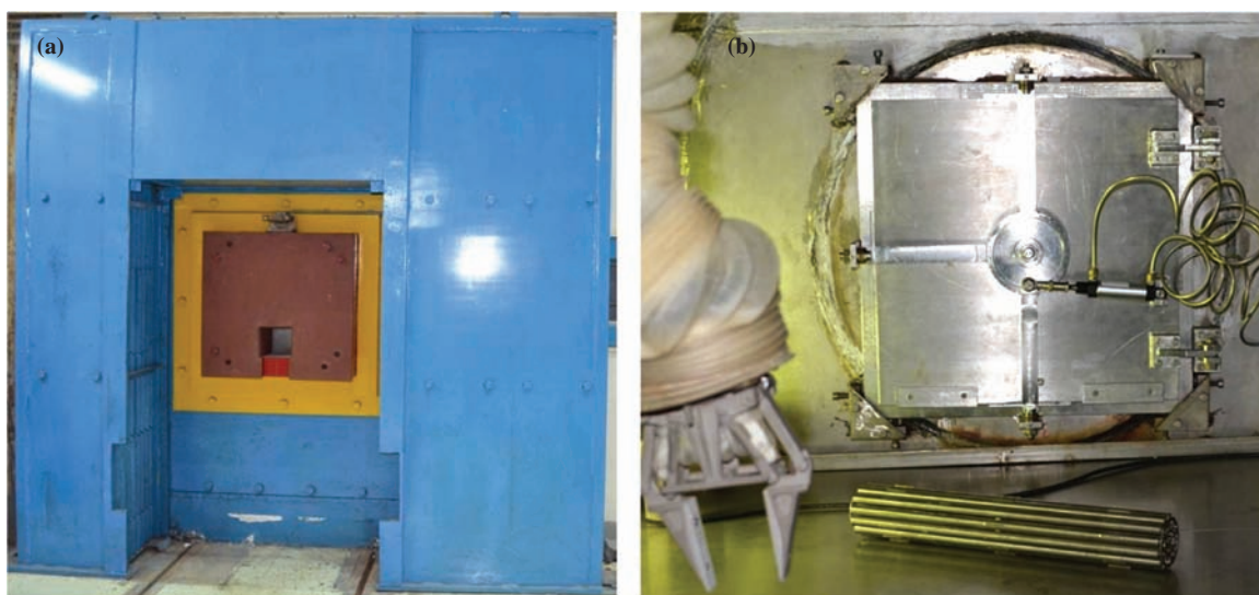
Fig. 2: (a) Cold side and (b) hot side of the transfer port in the new hot cell
