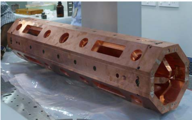
Fig. 7: RFQ assembly after 1st stage brazing
