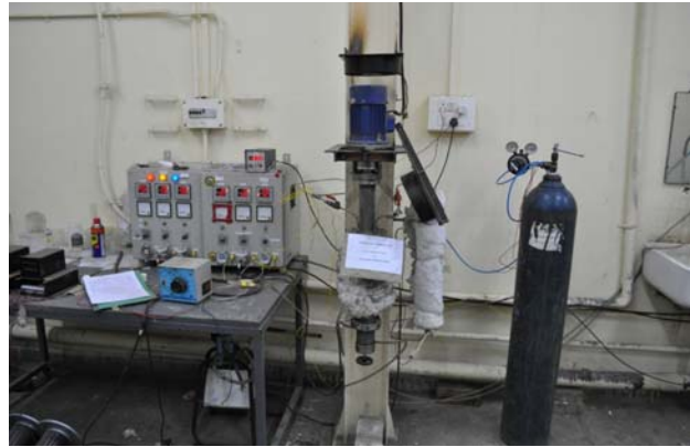
Fig 4:- Rotating disc Corrosion test facility
