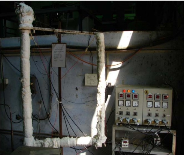
Fig. 1: The first Buoyancy Loop installed with Pb-17Li
