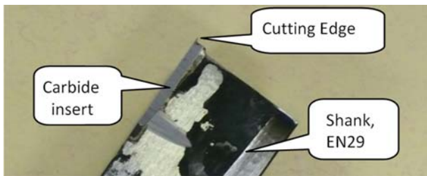
Fig. 4a: Tool for 17-4-PH Steel; Carbide insert brazed in SS EN29 shank.
