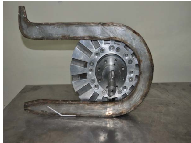
Fig 2: Sectional View of the Electromagnetic Pump.
