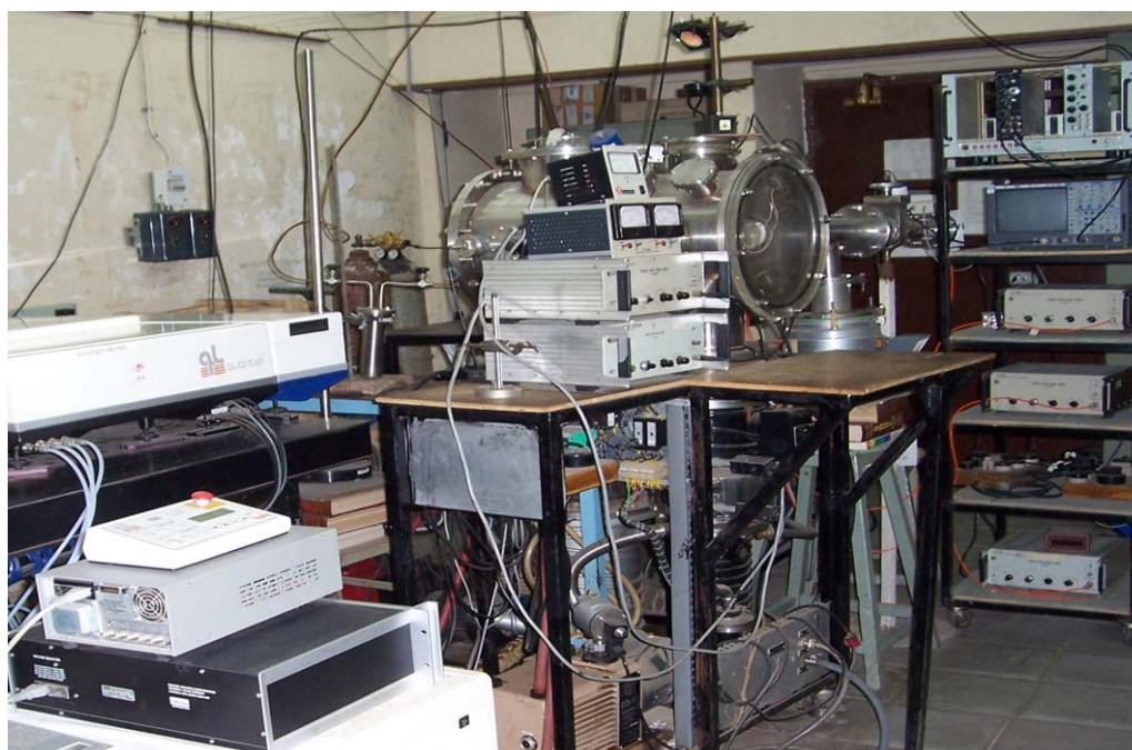
Fig. 1: Experimental setup for in-situ generation and photoionisation studies of cluster (indigenously designed and fabricated at BARC)
