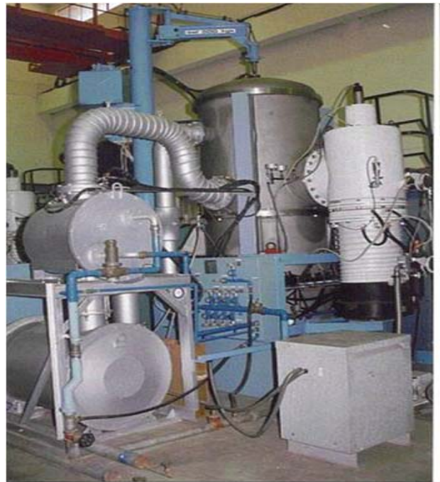
Fig. 6: Overall view of vertical vacuum furnace
