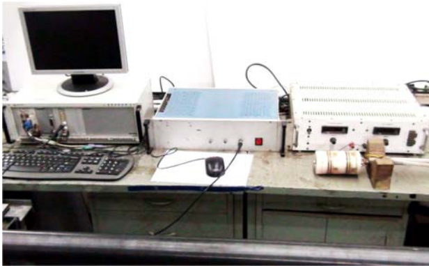
Fig. 3: Pulsed Eddy Current System for Garter Spring Detection.
