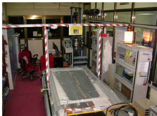
Fig.8, Facility for leak and spacer test of the bakelite gas-gaps at NPD-BARC
