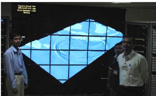
Fig. 1: Tsunami simulation using the LCD based 6x6 tiled display system.
