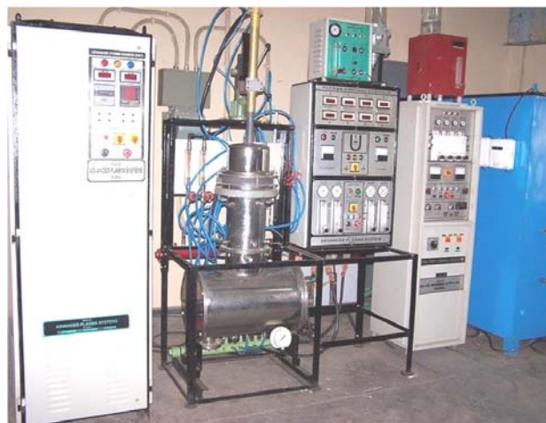
Fig. 7: 40 kW plasma reactor for nano-material synthesis
