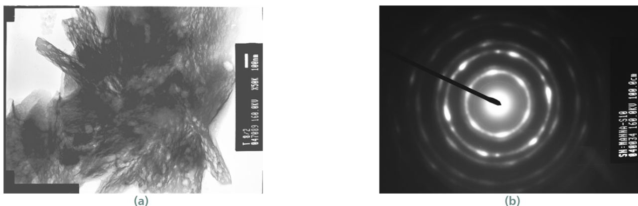
Fig. 3: TEM images of final ADU a) microstructure, b) selected area diffraction pattern
