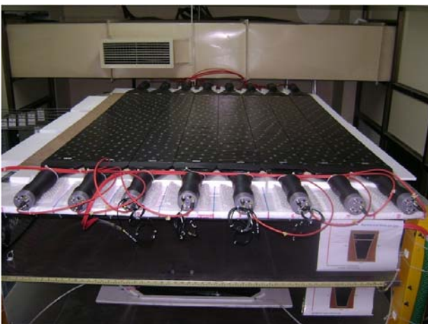
Fig.7: The top layer of scintillators (each 2m long) on the hodoscope for providing the muon trigger
