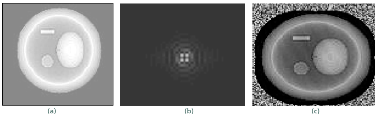
Fig. 7 (a) Simulated exit wavefield of cell containing lipid membrane and protein (b) its far-field diffraction pattern (c) Reconstructed object from the diffraction pattern
