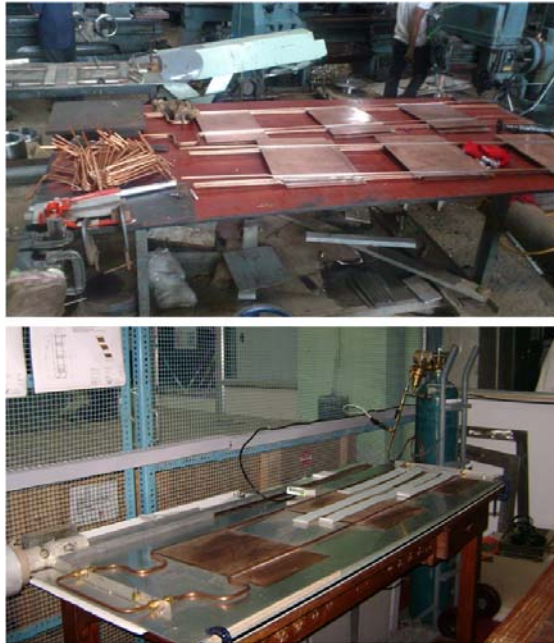
Fig.15: Mass production of Cu cooling assemblies (top) and a typical RE4/3 cooling set under leak test at NPD-BARC (bottom)
