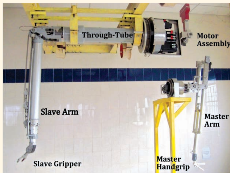
Four-Piece Servo Manipulator and its components
