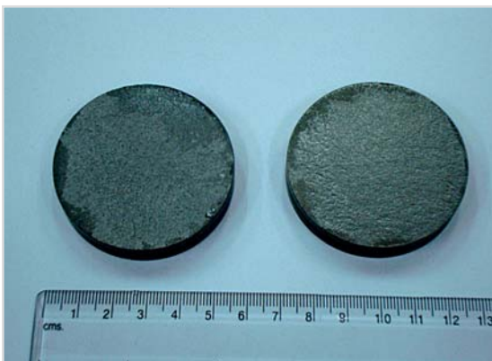
Fig. 5: \beta -FeSi 2 blocks prepared by the new route
