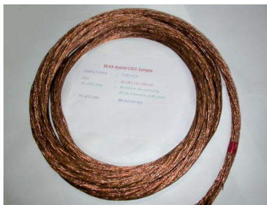
Fig. 5: Final Stage Cable Containing 504 wires of 0.8 mm dia
