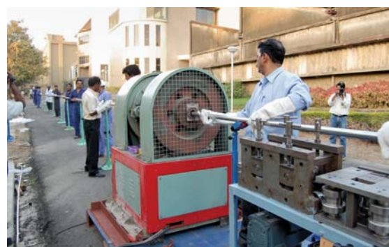
Fig. 10: Swaging of SS316LN tube containing cable to Square cross section CICC
