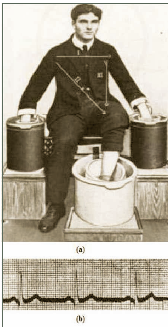
Fig. 1: Shows the beginning of the recording of an electrocardiogram. Saline tanks are used as electrodes as shown in (a); the ECG obtained with the help of string Galvanometer is shown in (b) (courtesy Einthoven W. 1901).
