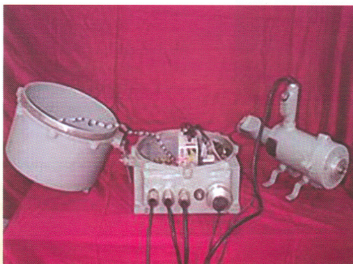
Fig. 6: Drive Motor with the Controller (explosion-proof construction)
