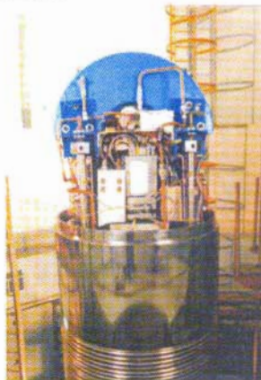
Fig 4 180°-folding magnet inside the high voltage terminal
