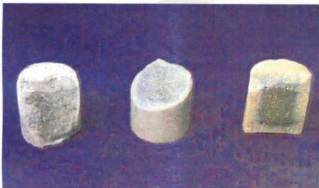
Fig. 3a TBO pellets with high sulphur shattered during drying
