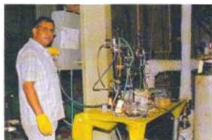
Fig.4 Sampling Station and On-line Dissolved Oxygen measurement facility
