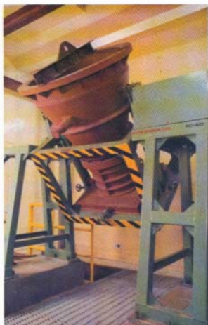
Fig. 3 Discharging stand for MTR reactor
