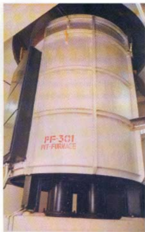
Fig. 2 Pit furnace for reduction
