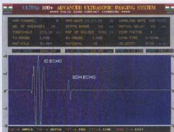
Fig. 5 A-scan at 1.5mm dia. SDH location
