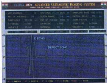
Fig. 8 A-scan at natural defect location
