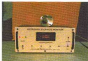
Fig. 4 Photograph of H_2S monitor showing sensor head and control unit.
