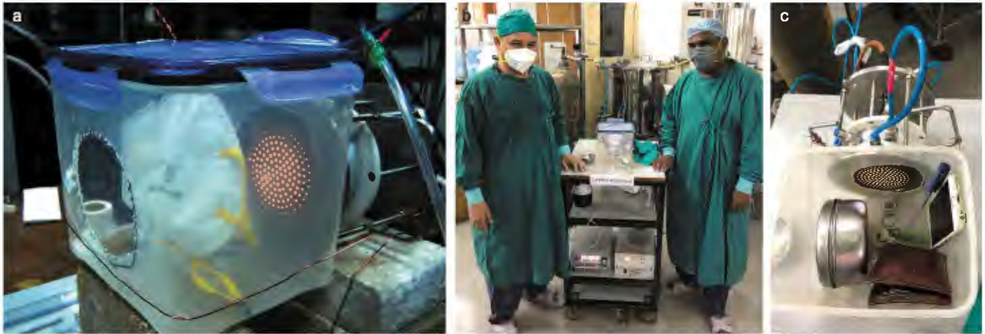
(a) N-95 mask being treated under Cold plasma (b) Cold plasma disinfection set-up in BARC Hospital, (c) Disinfection of personal belongings under cold plasma treatment in BARC Hospital.
