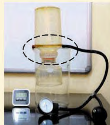
Synthetic Blood Penetration Resistance Test setup
