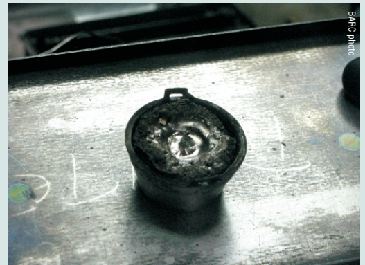
Metallic oxide layer formed at the surface for Tin
