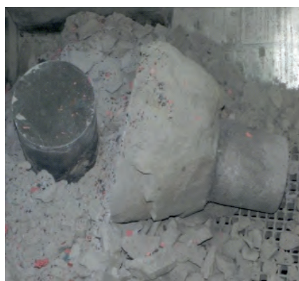
Fig. 6: NG-U metal ingot produced from SDU
