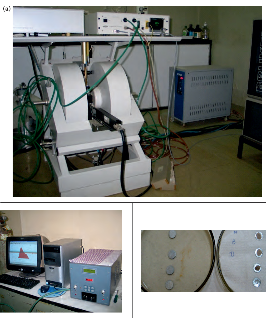
Fig. 1. a) Experimental set-up of the EPR spectrometer, (b) Experimental setup for TL measurements and the aluminium discs with isolated minerals from food samples for TL study
