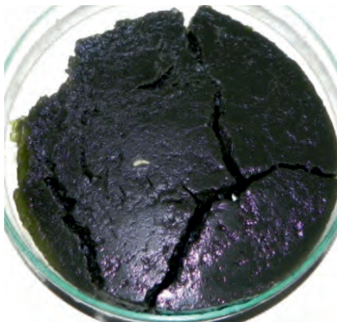
Fig. 3: Gelatinous cake obtained after acid dissolution
