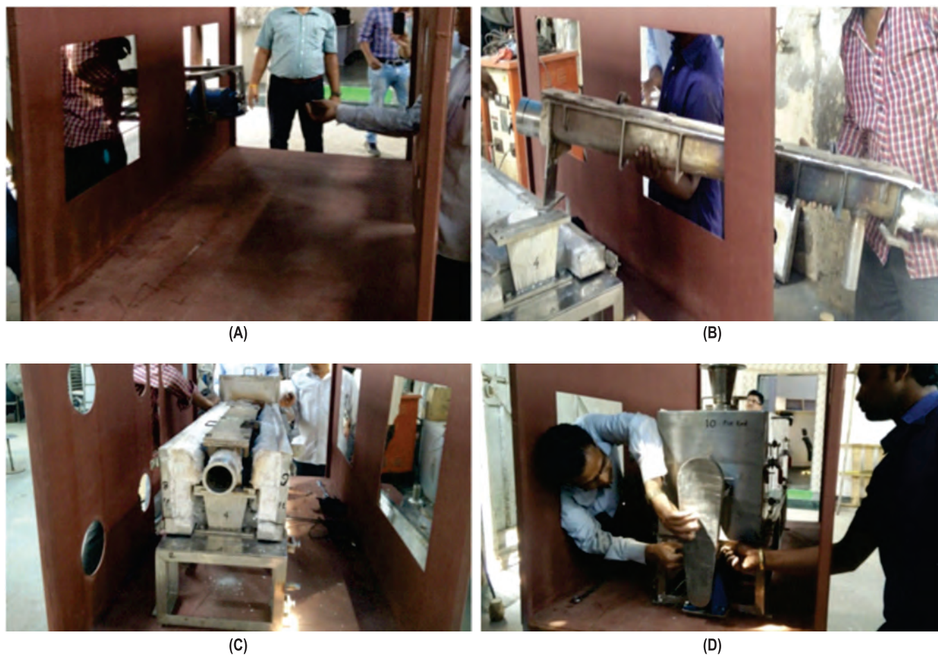
Fig. 11(A-D) : Assembly of RSC inside Dummy Glove Box
