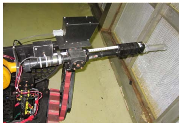
Fig. 2: Robot scanning HEPA Filter bank at WIP, Trombay
