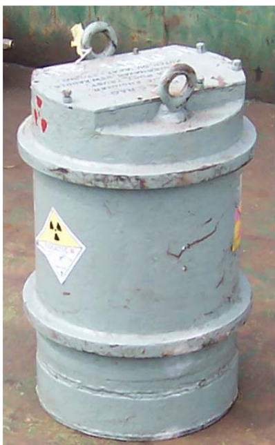
Fig. 2: Lead container used for transportation of radiotracer
