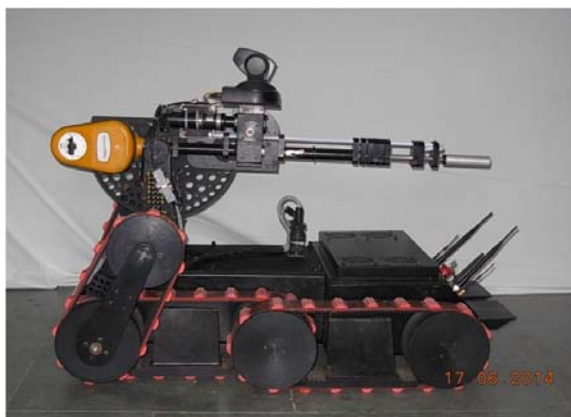
Fig. 1: All Terrain Robot with Retractable Radiation Detector
