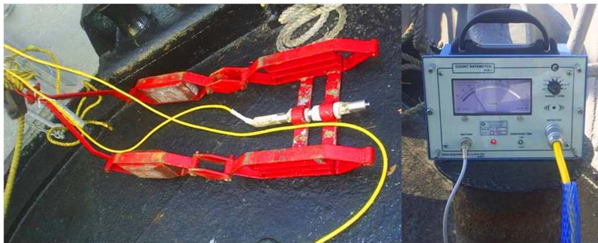
Fig. 4: Sledge mounted with a radiation detector and ratemeter used for monitoring of radiotracer
