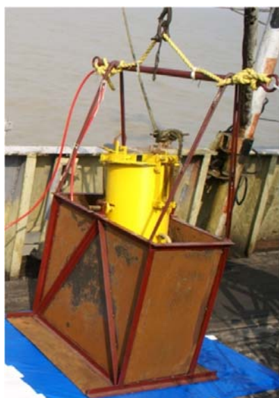
Fig. 3: Radiotracer injection system
