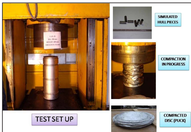
Fig. 3: Compaction tests at 1000 Te CDCFT press
