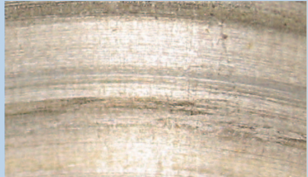
Fig 3 (b) : 22210CC Outer race wear out
