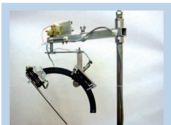
Fig. 12: Alternative robot configuration for endoscope control
