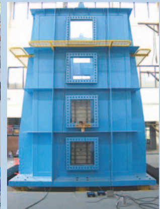
Fig.10: Spent Fuel Storage Pool loaded on the 25 ton shake table
