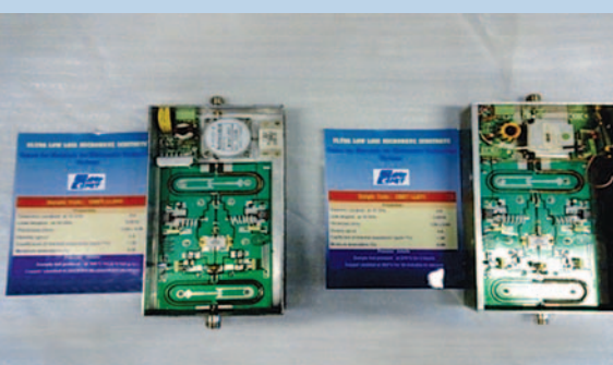
Fig.7 : Prototype high power solid state amplifiers fabricated at RRCAT, Indore
