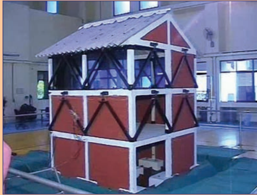
Fig. 7: Structure without FRP retrofit
