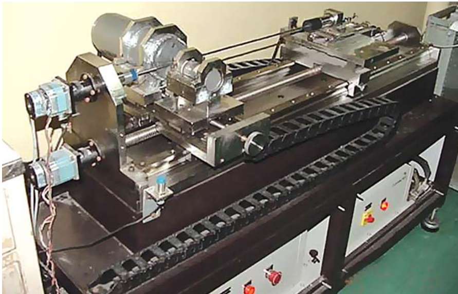
Fig. 6 : Gamma scanning system with detector and source moving simultaneously. The pin can be rotated at variable speeds.
