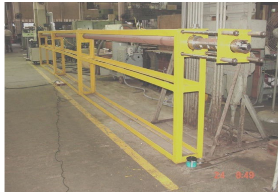
Fig.1 Separator / sensor tip cutting machine
