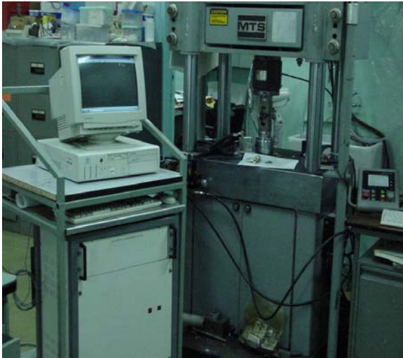
Fig. 2 DCPD unit connected with a servohydraulic test frame for fracture testing.
