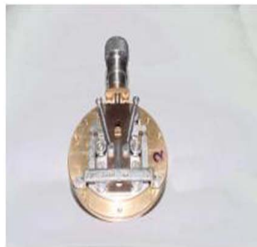
Fig. 4 Internal details of variable opening slit
