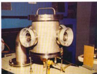
Fig.3. Spectroscopic sources developed for high resolution spectroscopy related to the clean-up programme. These sources work with milli to microgram quantities of isotopes of interest. Top: Hollow cathode discharge sources for emission spectroscopy and laser spectroscopy. Bottom: Atomic beam source for high resolution fluorescence spectroscopy.
