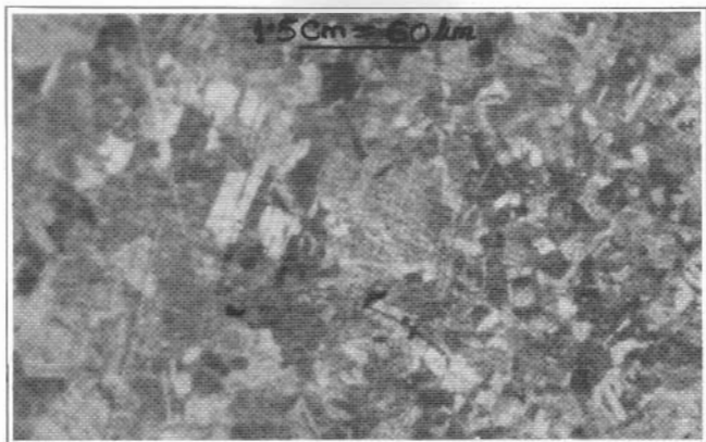
Fig. 3 Micro-structure in specimen no. 4 (welded at 100 cm/min.)
