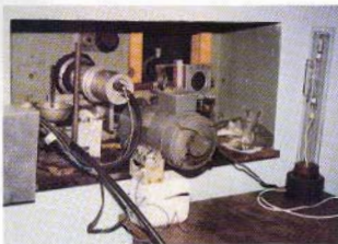
Fig. 3. View of REFPOS Facility. Left : Entrance slit of high resolution monochromator with detector. Right: Fabry Perot assembly with detector.
