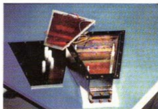
Fig. 3 \Delta E_{\mu} - E_{\mu} Position sensitive ionization chamber.
