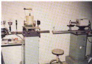
Fig. 3. View of REFPOS Facility. Left : Entrance slit of high resolution monochromator with detector. Right: Fabry Perot assembly with detector.
