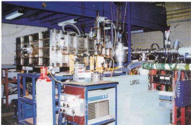
Fig.8 Large Area Position Sensitive Ionization Chamber
