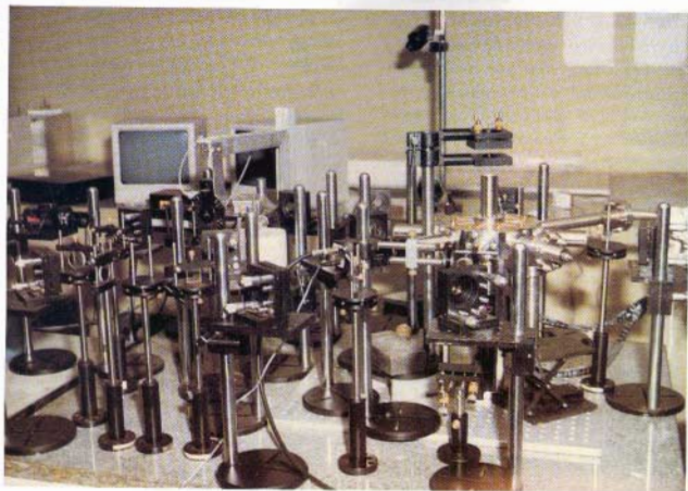
Fig.10. A view of the magneto-optical trap designed and developed in BARC.
