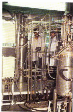
Fig 4 A 100 lit bioreactor successfully commissioned at Kabra Drugs Limited, Indore.
